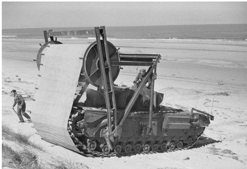
Above: Churchill AVRE (Armoured Vehicle Royal Engineers) Type C Mark II carpetlayer for laying tracks across soft beaches (IWM H 37859). Below: AVRE with spigot armament. Bottom: AVRE with SBG.
